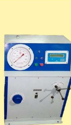
Digital Compression Testing Machine with Pillar Nut Type with extra fitted pressure gauge
